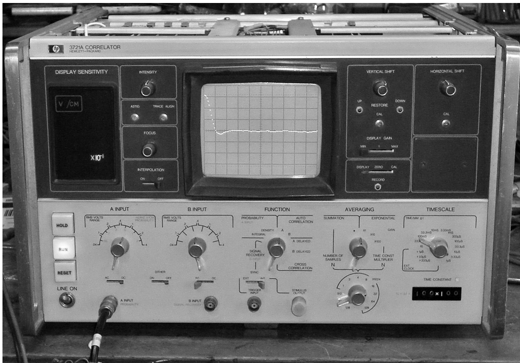
The preserved 3721A Correlator displaying the autocorrelation function of the 3722A Noise Generator
