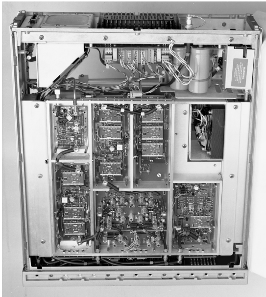
Interior showing hybrid amplifiers and filters
